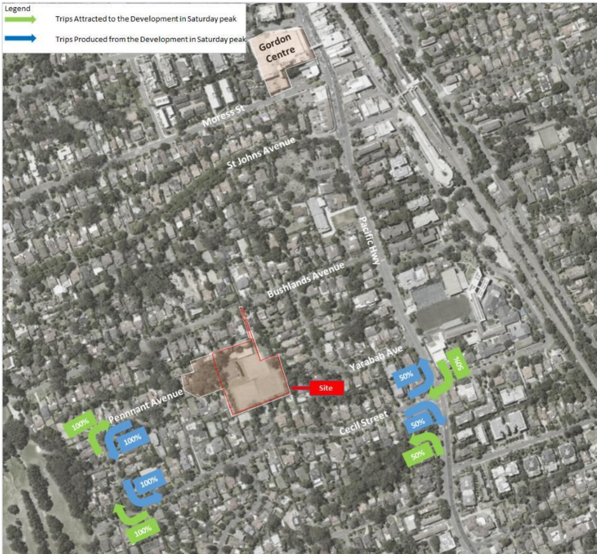
Figure 4-5 Trip Distribution Assumptions for Future Development Site at intersections of Pacific Highway/ Cecil Street in Saturday peak
